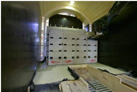
Stacking of test blocks in full scale
