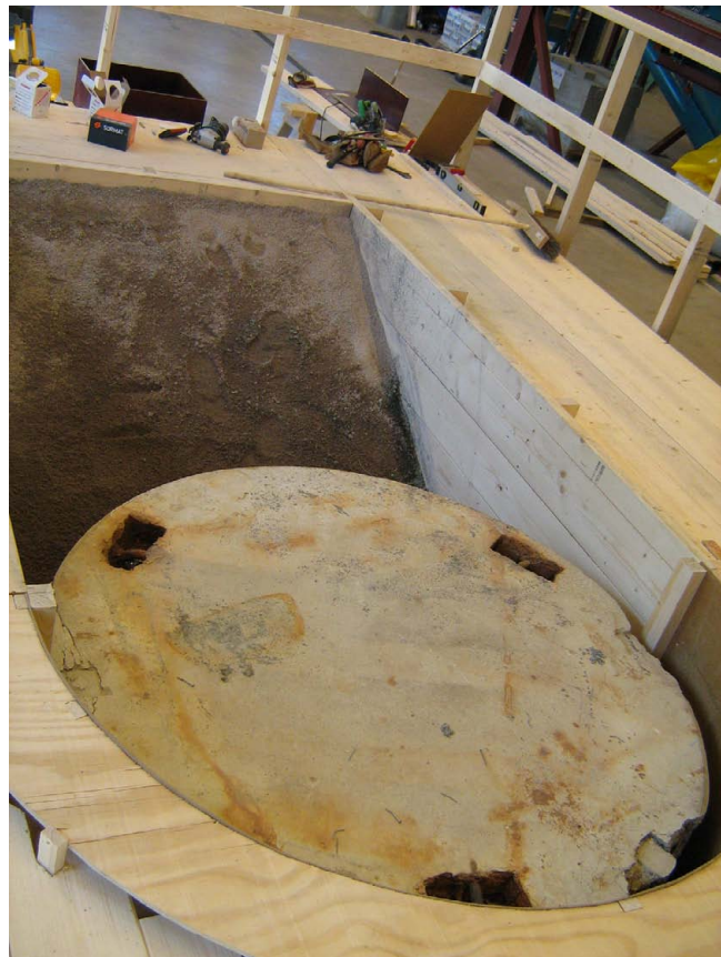
Figure 5-3. Test of backfilling of chamfer in deposition hole.
