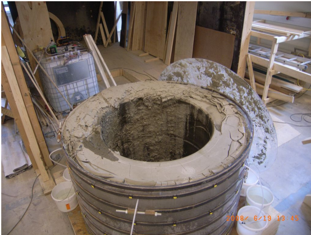
Figure 5-1. Piping and erosion test in the Bentonite Laboratory.
