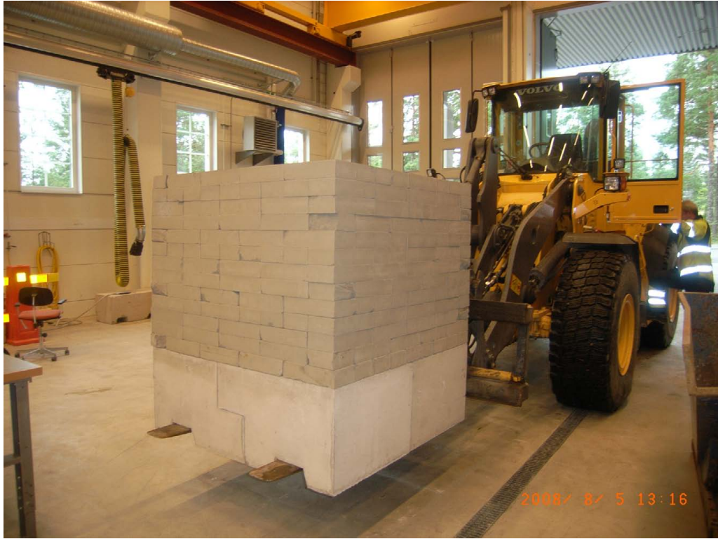
Figure 5-2. Module stability test.
