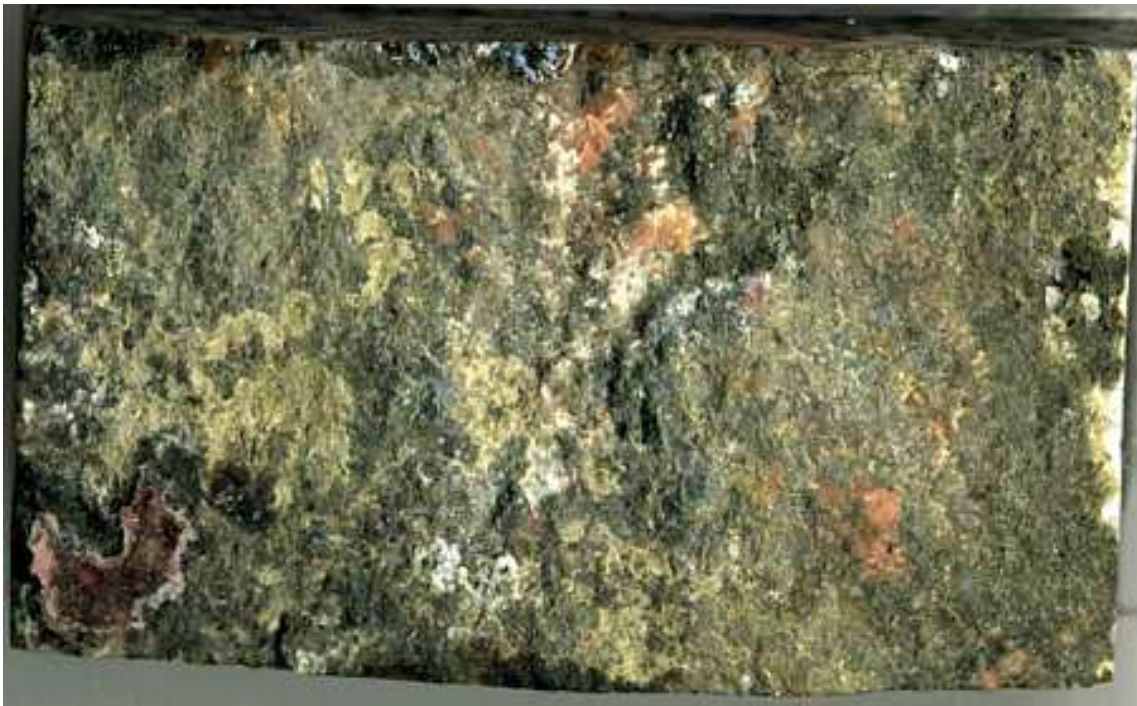
Figure 3-1. Fracture surface with thin coating of mainly chlorite, calcite, clay minerals and epidote. The length of the base of the photograph is 46 mm.
