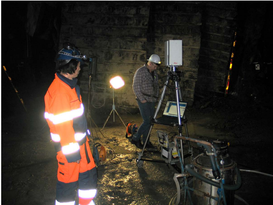
The first laser scanning session of the Tass-tunnel. The Leica scanner and a computer on the tripod.
